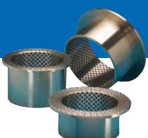
LUBRON® AQ self-lubricating bearings are widely used in offshore marine applications where environmental conditions are often severe, and external lubrication is impractical. LUBRON AQ bearings are constructed of corrosion resistant bearing alloys and permanent solid lubricants specifically developed for seawater use. LUBRON AQ bearings provide dependable performance and long life, require no supplementary lubrication, and are completely maintenance-free.
